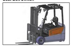
The seat belt switch is located next to the operator's seat.
