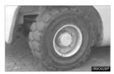
6. Install the steer wheel. Put two nuts opposite each other (180°). Tighten both. Install all remaining nuts. Tighten all nuts in a crisscross sequence opposite each other (180°) to a torque of 140 N·m (105 lb·ft).
