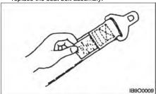
2. Belt Maintenance – Every 500 service hours. Check that the belt fastening works properly and that winding device is free from run lock when jerked. Check that the belt is suitably fastened to the seat. Check that the seat is correctly secured to the hood and the chassis. On visual inspection, fastenings must be intact, otherwise, contact the safety manager.
