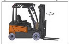
1. Tilt the mast to the full forward position.
