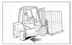
Do not drive in forward direction when loads restrict your visibility. Operate your lift truck in reverse to improve visibility except when moving up a ramp.
