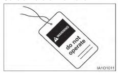
Attach a "Do Not Operate" or similar warning tag to start switch or controls before servicing or repairing the lift truck.
