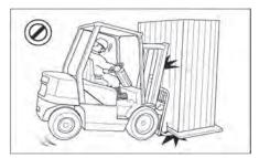
Do not overload. Always handle loads within the rated capacity shown on the capacity plate.
