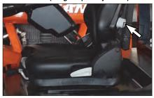
Turn the lumbar support adjusting lever to the right or left to tilt it backward or forward.
