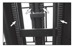
**6.** Inspect the chain anchors and individual links for wear, loose pins or cracked leaves.
