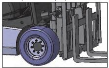
Park the lift truck on a level ground. Check that the parking brake lamp is on, and shift the control lever to the neutral position.
