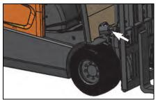
Inspect the hydraulic system for leaks, worn hoses or damaged lines.
