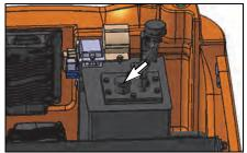
Drain the hydraulic system and fill it with SAE 5 or ISO VG 15, MIL-H-5606A hydraulic oil
