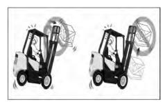
Do not elevate the load with the mast tilted forward.
