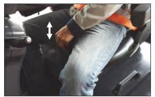
Pulling the weight adjusting lever forward by turning, move it up or down to adjust the weight input based on your weight (50–170 kg).
