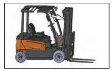
4. Tilt the mast forward and lower forks to the floor.
