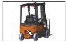
Lubricate fitting on steer axle.
