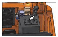
Loosen the bolts of the hydraulic tank top plate assembly.
