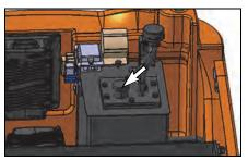
3. Remove an discard the hydraulic filter.
