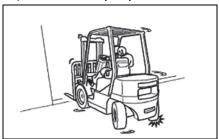
An unloaded forklift may be easier to tip over than a loaded truck.
