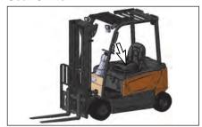
the seat switch is located under the operator's seat.
