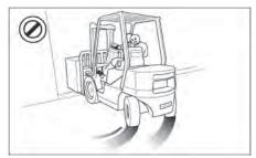
Do not start, stop, turn or change direction suddenly or at high speed. Sudden movement can cause the lift truck to tip over. Slow the speed of your truck and use the horn near corners, exits, entrances, and near people.
