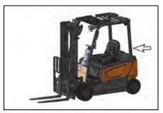
Inspect the overhead guard for damage, loose or missing mounting bolts.
