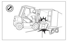
Do not operate on bridge plates unless they can support the weight of the truck and load. Make sure that they are correctly positioned. Put blocks on the vehicle you enter to keep it from moving.
